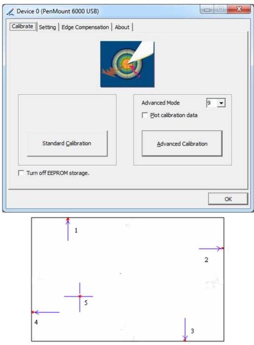
Step 2. Click "Standard Calibration" to start calibration procedure
