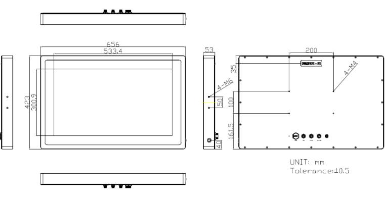
Figure 1.8: Dimensions of ViTAM-124P/G/(H)
